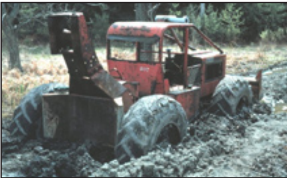
Rutting and soil compaction
